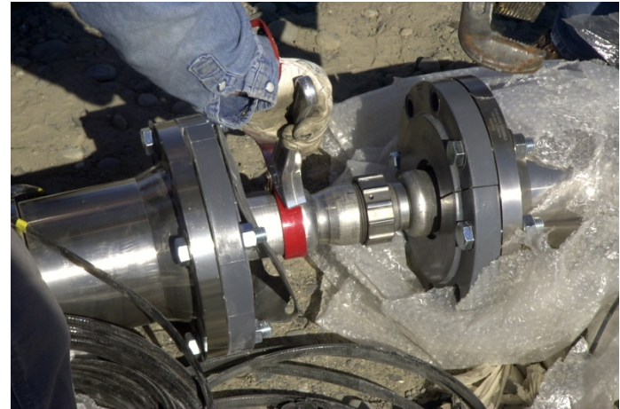
“Zero-clearance” fitting* for joining hose segments.
