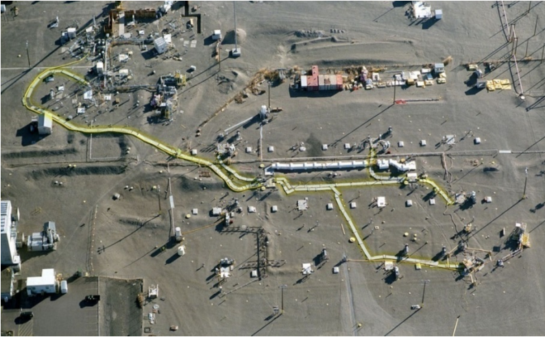
Multiple HIHTLs in DOE Hanford S & SY Tank Farms
